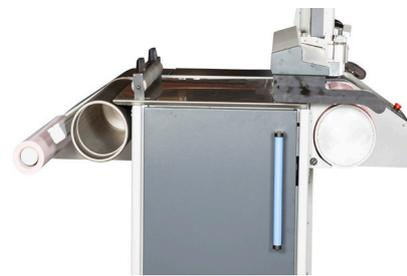
Tape roller integrated with cutting bar. Press roller for tape and plate material.
